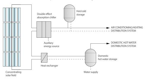
FLT can be also used in combination with ammonia-water absorption chillers, which are suitable for hot and arid climates thanks to their dry recooling and for cooling temperatures below 0°C. Furthermore, by using clean and renewable solar energy, concentrating collectors such as FLT represent the most appropriate technology for realising solar district heating and cooling systems.
